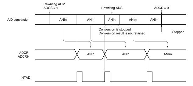
Figure 10-12. A/D Conversion Operation
