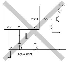
Figure 5-7. Examples of Incorrect Resonator Connection (2/2)
