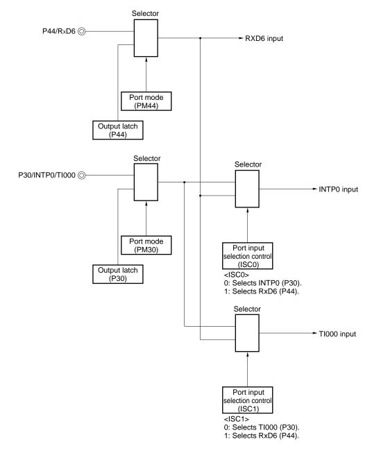
Figure 11-3. Port Configuration for LIN Reception Operation
