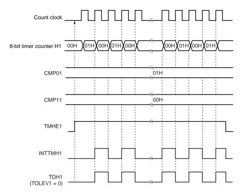
Figure 8-9. Operation Timing in PWM Output Mode (4/4)
