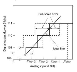
Figure 10-18. Differential Linearity Error
