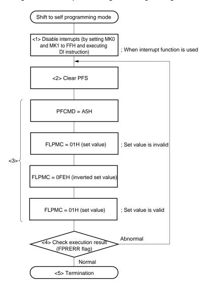
Figure 18-20. Example of Shifting to Self Programming Mode
