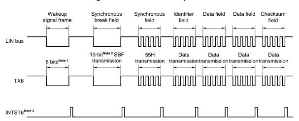
Figure 11-1. LIN Transmission Operation
