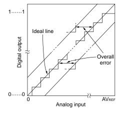
Figure 10-14. Quantization Error
