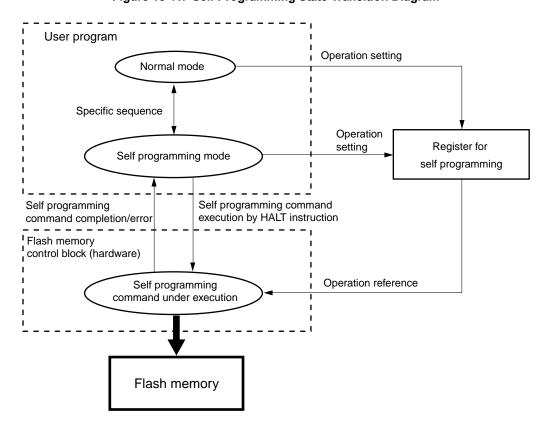
Figure 18-11. Self Programming State Transition Diagram
