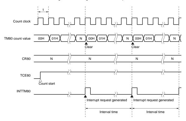
Figure 7-5. Timing of Interval Timer Operation
