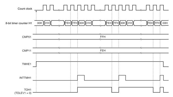
Figure 8-9. Operation Timing in PWM Output Mode (3/4)
