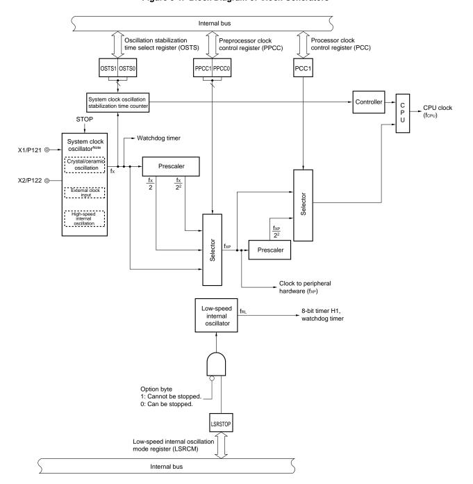
Figure 5-1. Block Diagram of Clock Generators
