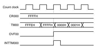
Figure 6-37. Operation Timing of OVF00 Flag
