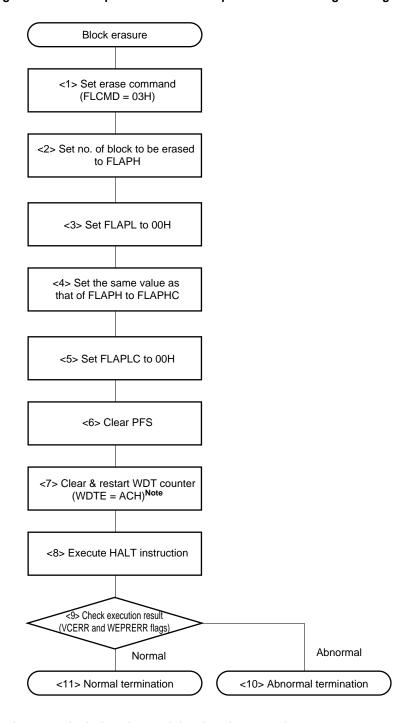
Figure 18-22. Example of Block Erase Operation in Self Programming Mode
