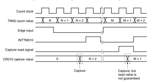
Figure 6-38. Capture Register Data Retention Timing
