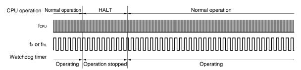
Figure 9-8. Operation in HALT Mode
