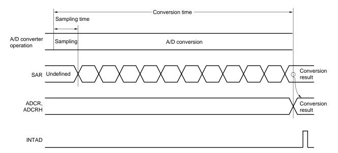
Figure 10-10. Basic Operation of A/D Converter
