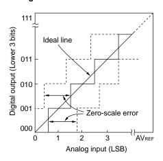
Figure 10-17. Integral Linearity Error
