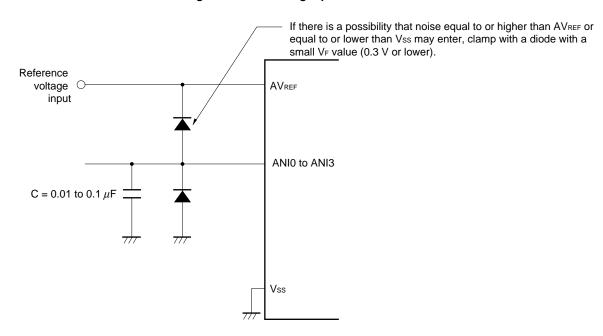
Figure 10-19. Analog Input Pin Connection
