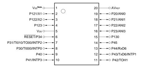
**Note** In the 78K0S/KA1+, Vss functions alternately as the ground potential of the A/D converter. Be sure to connect Vss to a stabilized GND (= 0 V).
