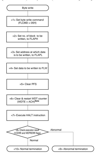
Figure 18-24. Example of Byte Write Operation in Self Programming Mode
