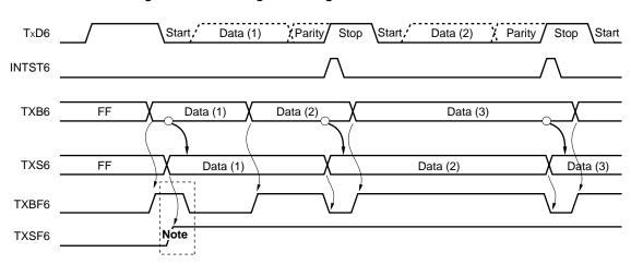
Figure 11-17. Timing of Starting Continuous Transmission
