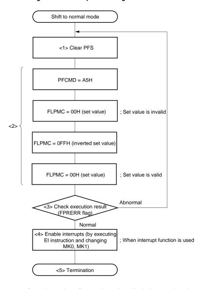
Figure 18-21. Example of Shifting to Normal Mode
