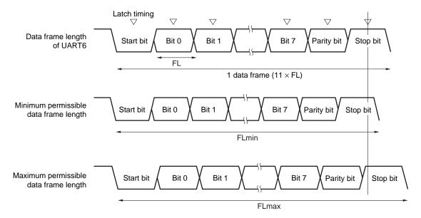
Figure 11-25. Permissible Baud Rate Range During Reception
