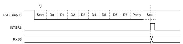
Figure 11-19. Reception Completion Interrupt Request Timing
