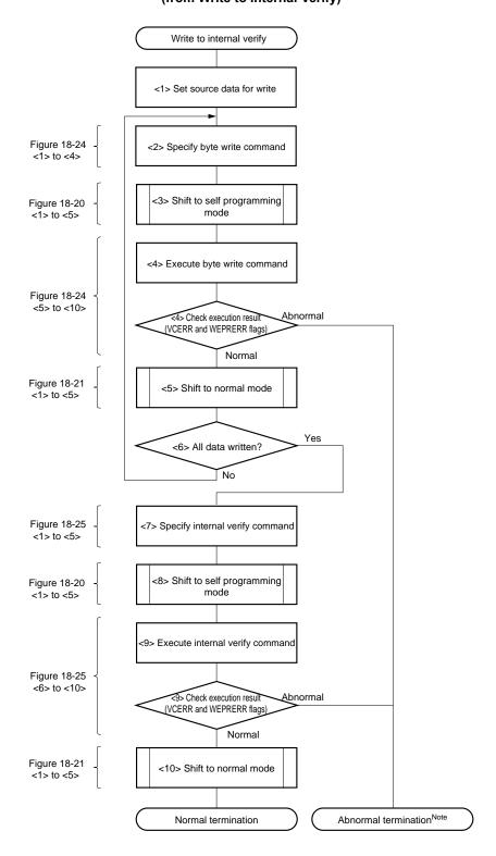
Figure 18-29. Example of Operation When Interrupt-Disabled Time Should Be Minimized (from Write to Internal Verify)
