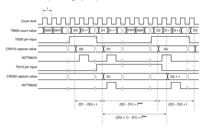
Figure 6-22. Timing of Pulse Width Measurement Operation with Free-Running Counter (with Both Edges Specified)
