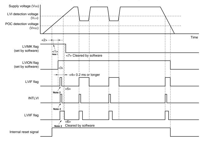
Figure 16-5. Timing of Low-Voltage Detector Interrupt Signal Generation
