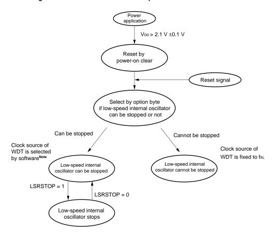
Figure 5-14. Status Transition of Low-Speed Internal Oscillation
