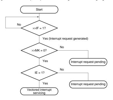
Figure 12-7. Interrupt Request Acknowledgment Processing Algorithm
