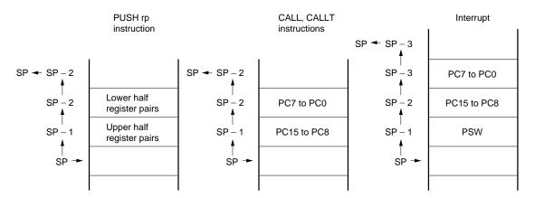
Figure 3-9. Data to Be Restored from Stack Memory
