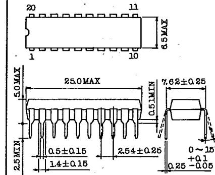
Lead pitch is 2.54 and tolerance is ±0.25 against theoretical center of each lead that is obtained on the basis of No.1 and No.20 leads.
