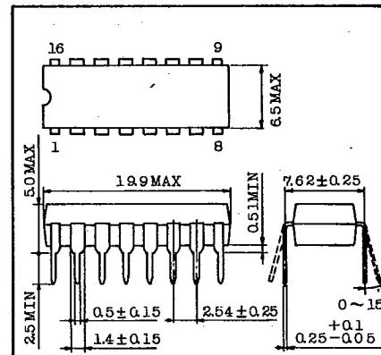
Lead pitch is 2.54 and tolerance is ±0.25 against theoretical center of each lead that is obtained on the basis of No.1 and No.16 leads.
