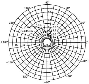
$S_{12e}$   $V_{CE} = 6V$   $I_{C} = 7mA$  $T_{a} = 25^{\circ}C$
