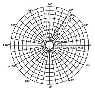
$\begin{array}{c} S_{22e} \\ V_{CE} = 6V \\ I_{C} = 3mA \\ T_{a} = 25^{\circ}C \\ (UNIT:\Omega) \\ \\ j_{25} \\ \\ -j_{10} \\ \\ -j_{25} \\ \\ \\ \\ -j_{50} \\ \end{array}$
